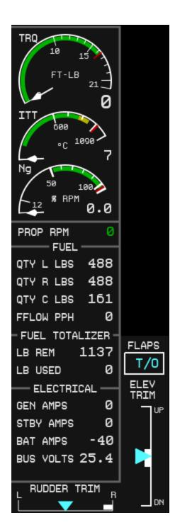
The System sidebar can be reached by pushing Softkey 1 on the MFD labeled "SYSTEM"
