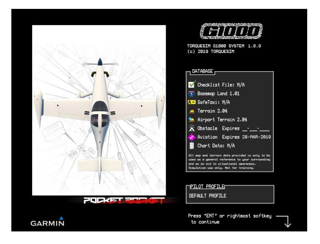
The screen shows the current expiration date for your Navigation Database, and the current version of the aircraft. Pressing Softkey 12 or the ENT key on the MFD will move to the G1000 moving map.
