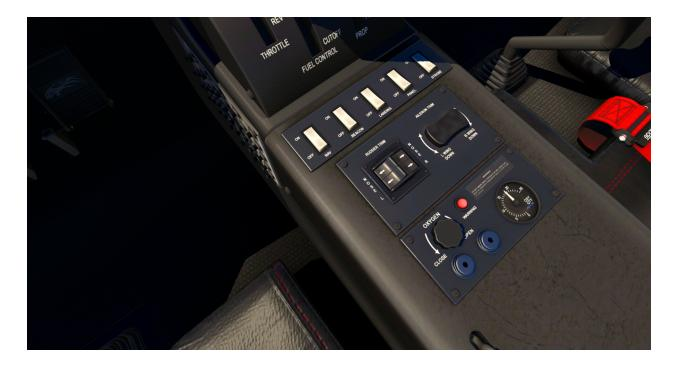
The oxygen system consists of a 2200 PSI oxygen bottle capable of dual operation for flights up to FL250. The oxygen bottle provides over 70 cubic feet of Oxygen storage. Turning the knob will enable the oxygen system. The red warning light is on whenever oxygen pressure is below limits or when the oxygen system is not delivering oxygen.
