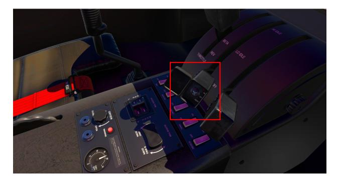
Clicking the switch up will engage the starter. The middle position is default. The down position will abort the start.
