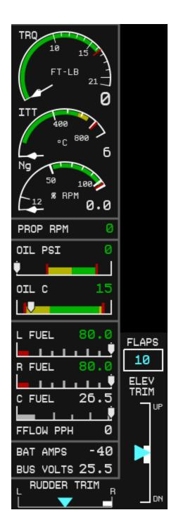
The engine sidebar presents the Torque, ITT, Ng, Prop RPM, Oil PSI, Oil Temp, L/R/C fuel (in gallons), Fuel Flow, Bat Amps, Bat Volts, Rudder Trim, Flaps, and Elevator Trim.
