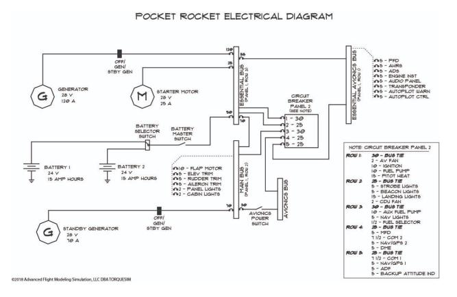
The electrical system consists of four electrical busses, the Essential Bus, the Main Bus, the Essential Avionics Bus, and Avionics Bus.
