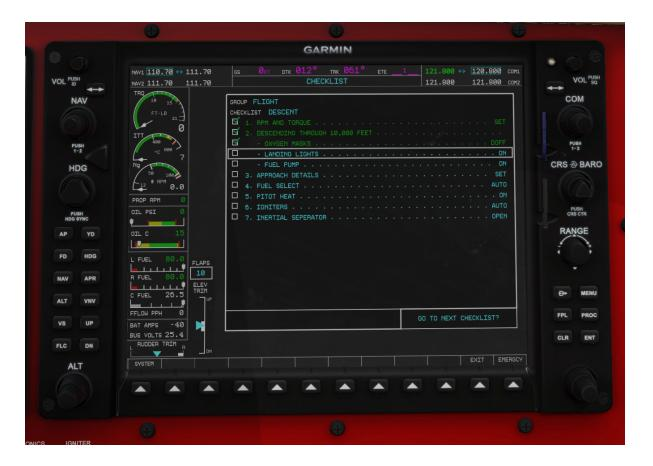
Checklists can be reached through softkey 11 on the MFD, labeled "CHKLIST". Clicking this will reach the checklist page. The outer FMS knob can be used to move the box cursor up and down. The inner FMS knob is used to control variable settings. The "ENT" key will check/uncheck the selected item and move to the next item on the list. The "CLR" key will clear the current checklist.
