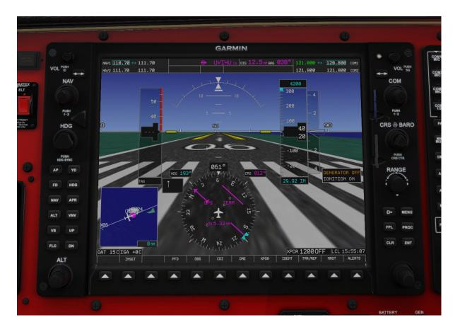
Synthetic Vision provides a 3D view of the space around you. You can control features of the synthetic vision through the "PFD" button (Softkey 4) and navigating into the "SYN VIS" menu (Softkey 1).
