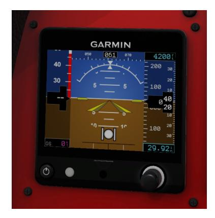
The G5 simulation is fully custom for the Pocket Rocket. It displays an airspeed tape on the left, magnetic compass at the top, altitude and vertical speed on the right, turn/slip indicator at the bottom, ground speed at the bottom left, baro pressure at the bottom right, altitude pre-select at the top right, and an attitude indicator in the middle.
